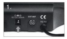
Connect the power adaptor to the antenna DC input.
